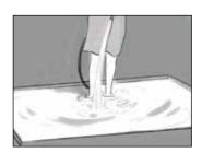
Remove it after 24 hours, and fill it up with water for flat surface; wrapping up for vertical member and curing to continue for 7 to 10 days
